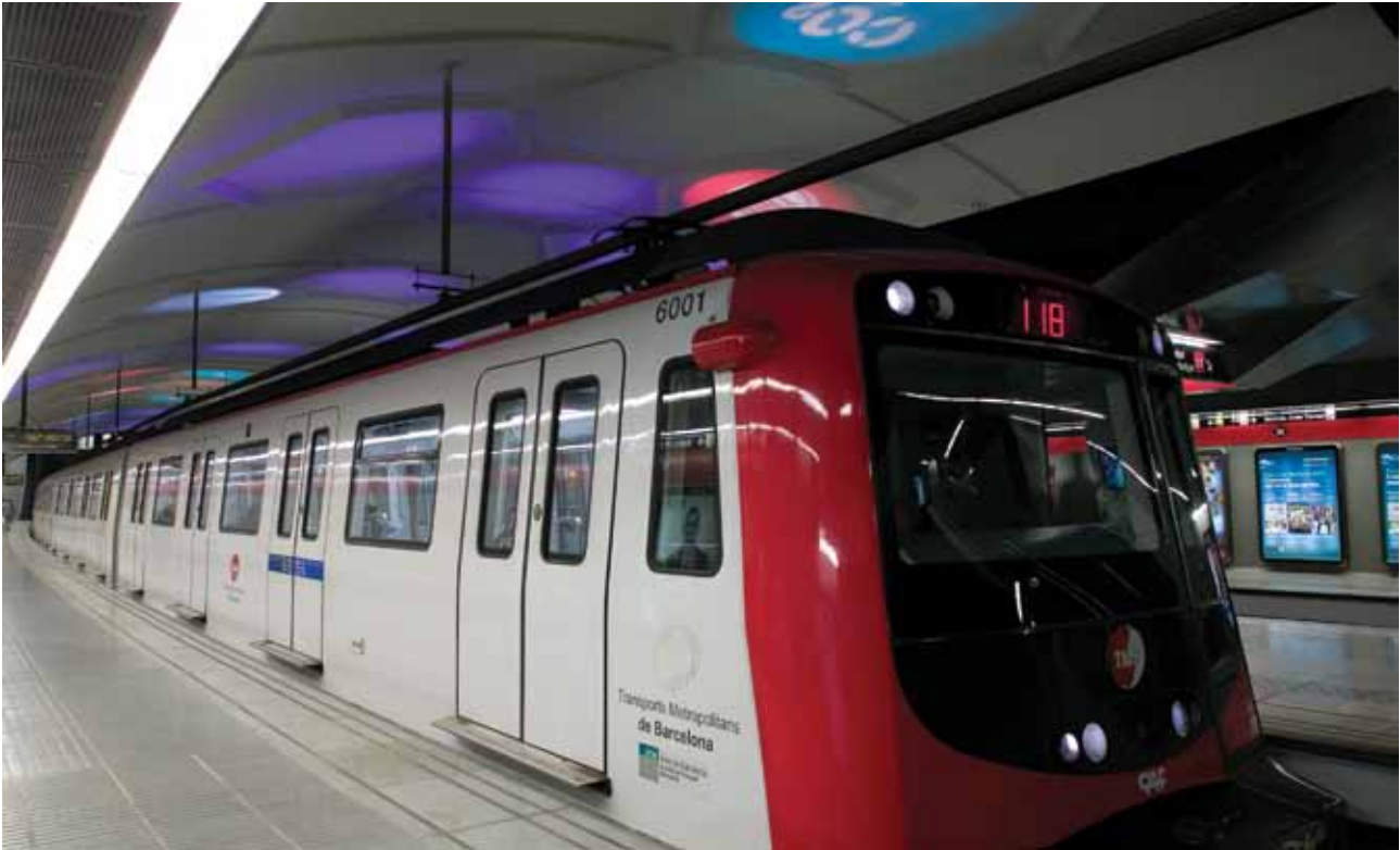
The system of spotlights and floodlights that is used to illuminate the vault allows for projections of advertisements or information campaigns, which alter with streams of light,color and movement. The goal is a constantly changing perception of the station by its users.
